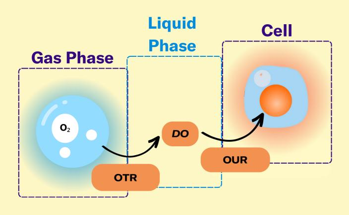
**Oxygen Transfer Rate (OTR)** refers to how fast oxygen molecules can move from a gas bubble to the liquid media. To do so,  $O_2$  molecules must diffuse through a stagnant region called the gas-liquid interface. The OTR is influenced by the volumetric mass transfer coefficient (kLa).
