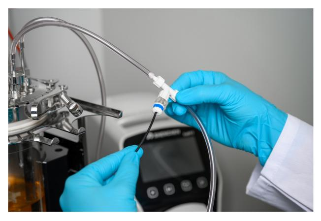
Continuously monitor dissolved oxygen (DO) in flow loops using fiber optic sensors.
