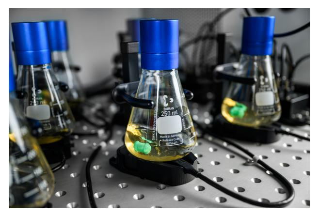
First pill-based optical sensor for online dissolved oxygen (DO) monitoring in shake flasks.
