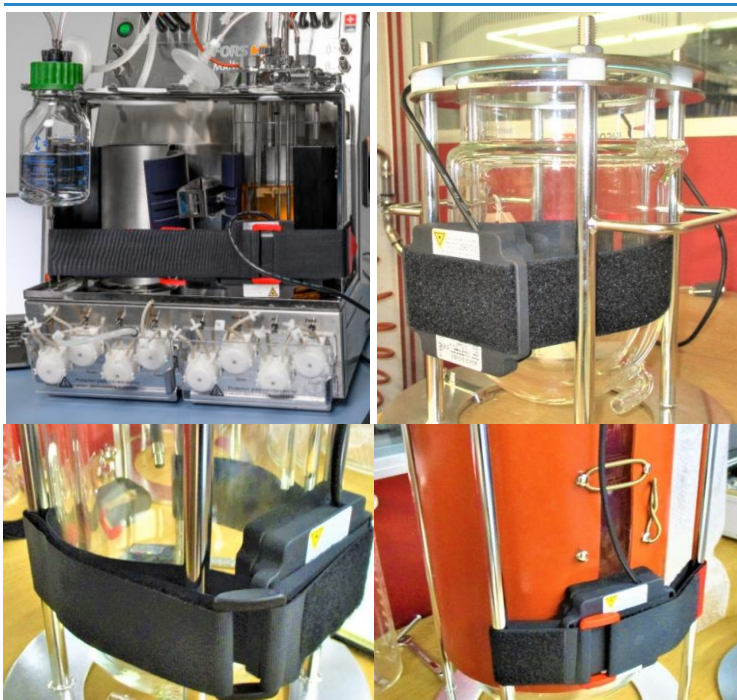
Figure 16: Exemplary setups of BioR Sensors mounted on bioreactors, mounting the belt around the complete bioreactor setup, around the vessel, around the vessel and rods and around two rods.
