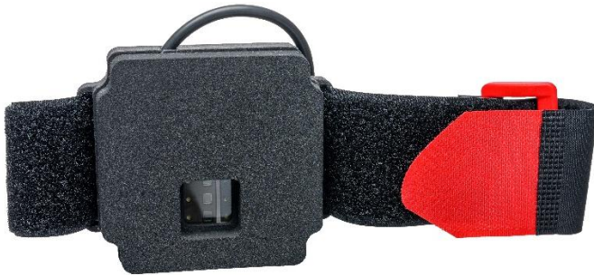
Figure 15: The BioR Sensor with elastic foam and Velcro belt.
