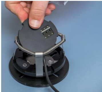
Figure 8: Mounting the CGQ in a Sensor Adapter – Step 1.
