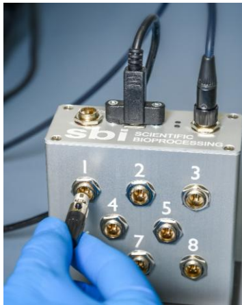
Figure 10: Connecting CGQ Sensors to the CGQ Hub.
