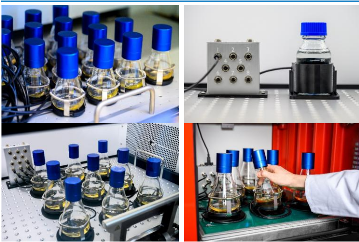
Figure 3: CGQ components assembled for Erlenmeyer flasks with Lauber clamps or Sticky Mat/Clamp Adapters and for bottles with Bottle Adapter.
