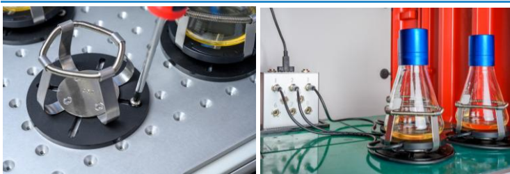
Figure 4: Mounting of Sticky Mat/Clamp Adapter on shaking tray with screwing threads (left) and sticky mat (right).
