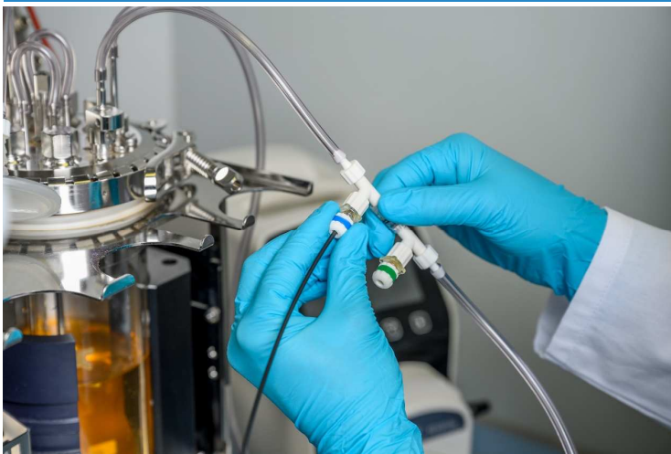
Figure 14: Connecting a fiber optic cable to an in-line DOTS Flow Cell.
