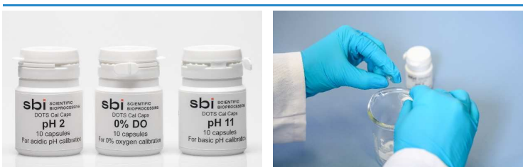
Figure 19: DOTS Cal Caps for preparing pH 2, pH 11, and 0% DO calibration solutions.
