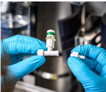
Figure 9: Replacing a Luer cap with a Luer-barb connector on a sterile, pH flow cell.
