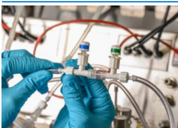
Figure 12: Connecting a DO and pH flow cell together within a sterile flow loop via a male-male Luer connector.
