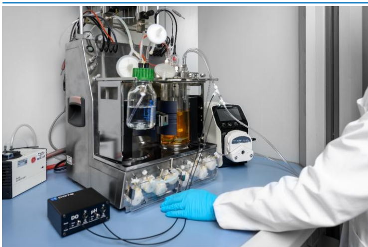
Figure 18: The DOTS Fiber Optic Sensor and DOTS Flow Cells connected in a bioreactor flow loop.
