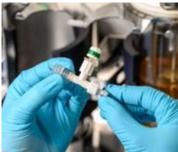
Figure 11: Replacing the remaining Luer cap from a pH flow cell with a dual-thread, male-male Luer connector.
