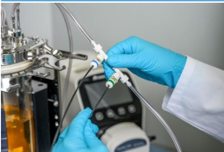
Figure 15: Completing the connection of two flow cells to the DOTS Fiber Optic Sensor via two fiber optic cables.
