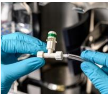
Figure 10: Connecting one side of a pH flow cell into a sterile flow loop.
