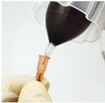
Figure 24: Filling the headspace of the sterile needle with liquid.
