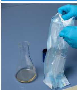
Figure 12: Assembling the LIS – Preparing the sterile Cartridge.
