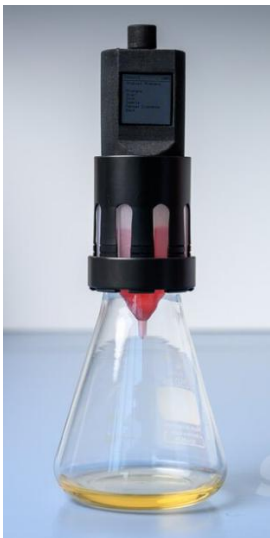
Figure 22: Preparing the LIS Drive – Replacing the LIS back onto the flask after removing the Luer plug.
