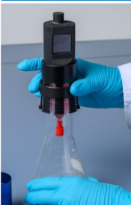
Figure 17: Assembling the LIS – Securing the Drive and Cartridge together by placing the Mounting System ring over the Octagrab.
