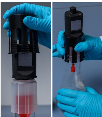
Figure 16: Assembling the LIS – Coupling the Drive with the Cartridge using the Octagrab.
