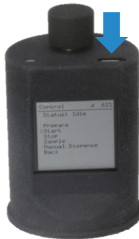
Figure 6: A powered-on LIS Drive with an arrow indicating the micro-USB charge port .
