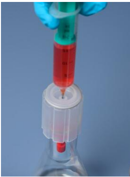
Figure 13: Assembling the LIS – Filling the Cartridge.
