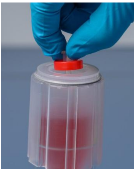
Figure 14: Assembling the LIS – Installing the sterile filter on the Cartridge.
