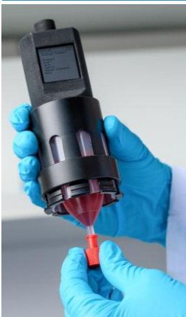
Figure 20: Preparing the LIS Drive – Removing the Luer plug.
