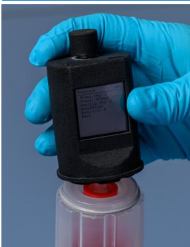
Figure 15: Assembling the LIS – Placing the Drive on the Cartridge.
