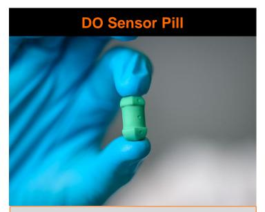
The single-use, factory-calibrated pill is simply dropped into the shake flask culture. Circulating with the medium, it measures dissolved oxygen continuously.
