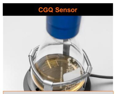
The sensors are positioned under the shake flasks and measure the biomass non-invasively.
