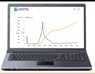
DOTS Software enables a simplified control of sensors and visualizes the received data from all monitored shake flasks in real-time.
