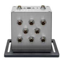
The base station bundles the data from all monitored bioreactors and sends it to the DOTS Software.
