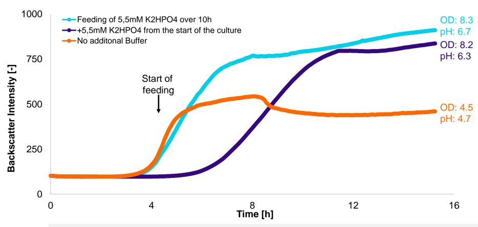
Escherichia coli, 25 mL LB Medium + 2% Glucose, 250 mL Shake Flask, 37°C, 250 rpm growth curves monitored with the CGQ
