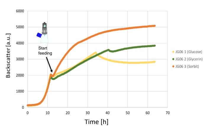
H. polymorpha grown on mineral medium, 180 rpm, 30°C. Feeding rate: 2.5 g/L\*h
